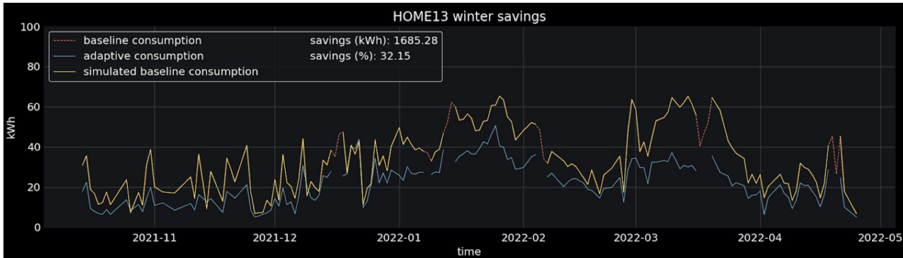
Real Adaptive + Simulated Baseline Consumption per day over the entire heating season
